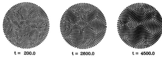
FIG. 1. Spontaneous formation of spirals from a random initial condition without non-Boussinesq effects and without lateral heating. If we fix the values for the temperature field on the sidewall, we obtain rolls parallel to the wall and spirals in the bulk. The essential mechanism for spiral formation is the influence of a large-scale mean flow, caused by the low Prandtl number (for details, see [8]).
